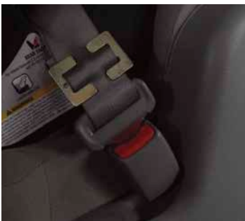
Locking clip used on a forward-facing car seat.
